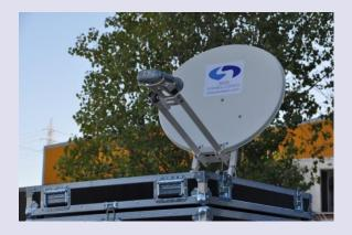
SVSATNM 78-Ka helps operator to find satellite with a user interface. Instead of motors, operator can find the desired satelite by adjusting to antenna reflector by looking to the computer screen. When satellite is found, the software warns you that it is "locked". The software also provides audio visual alarms.
